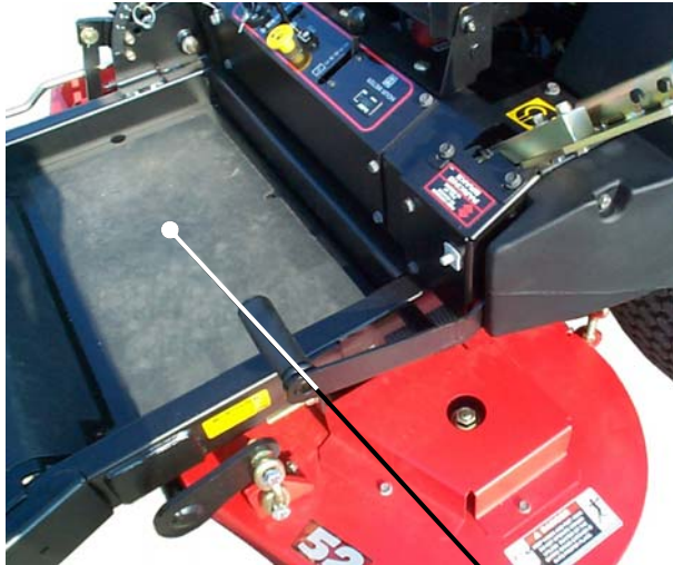
LIFT FOOT REST UP AND OFF POWER UNIT FRAME TO GAIN ACCESS TO MOWER BELT
