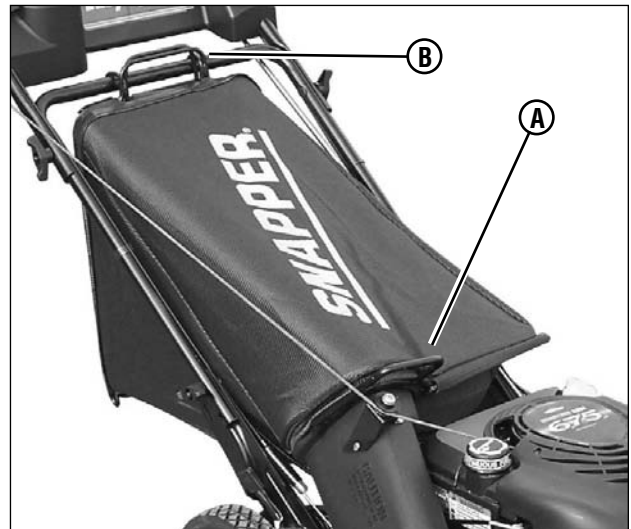
Figure 15: Installing the grass bag
