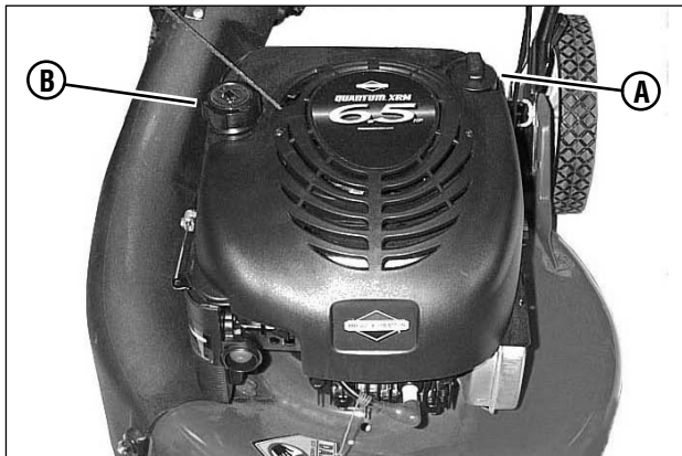
Figure 2: Oil and fuel fill
