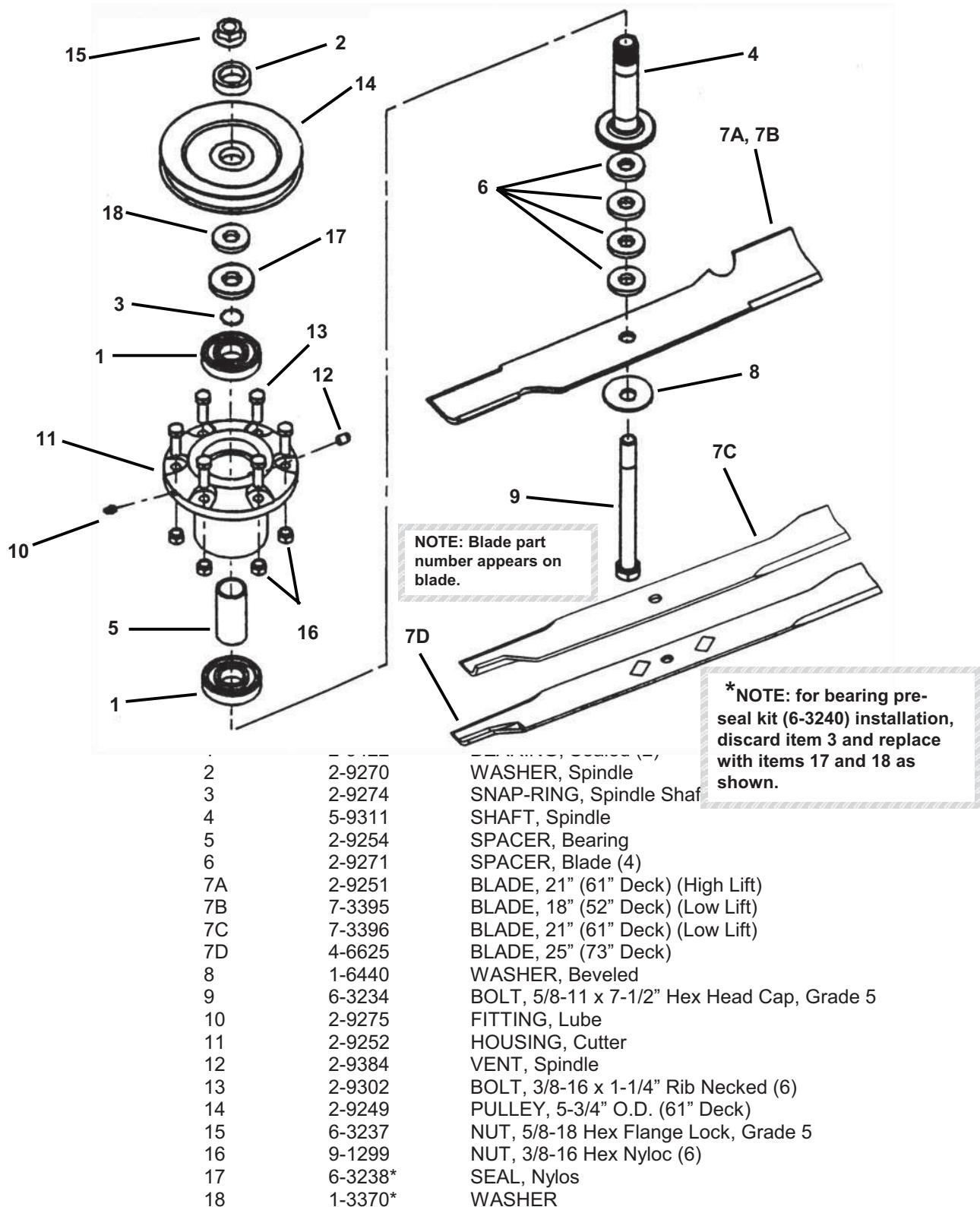
NOTE: Part Number 5-4017 (Spindle Housing sub-assembly) is comprised of items 11 and 12 (one each) as well as item 13 (six each).
